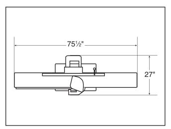
Figure 4. Model G0586 overhead dimensions.
